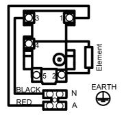
Connect the active and neutral wires to the terminal block and the earth wire to the earth tab (located on the right hand side). Excess wire is not to be looped close to the thermostat or tank.
